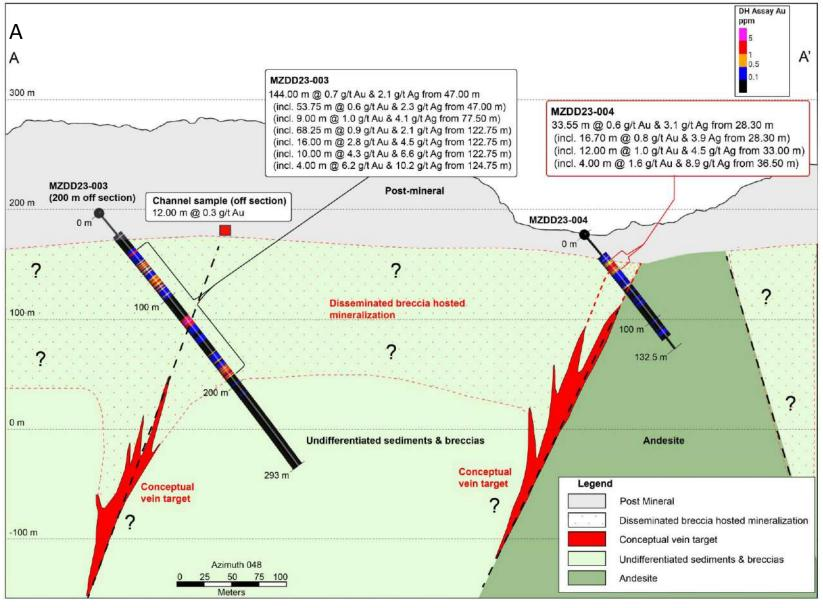
Next phase of drilling to test 100 – 200m below identified mineralization
